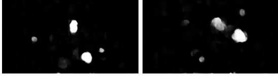
Fig. 8. U-Net outputs representing the probability of each pixel belonging to spiking neurons. The input temporal summary images are shown in Figure 5.
